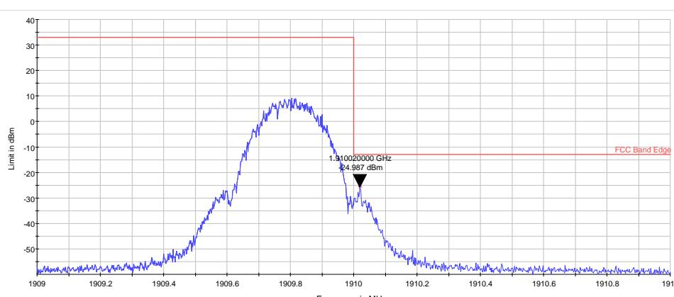
RMS (RBW: 3 kHz, VBW: 3 kHz, Max hold)
