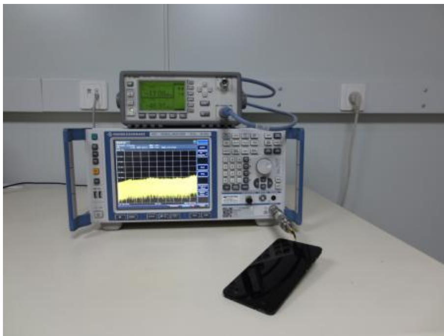
Spurious RF Conducted Emissions Test setup
