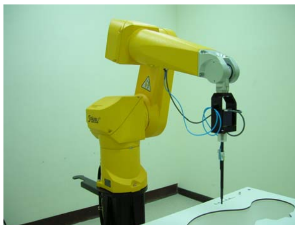
Fig. 5.2 Probe setup on robot
