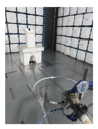
Photograph No.2 Setup for carrier and spurious emissions measurements in anechoic chamber from 30 MHz to 1 GHz
