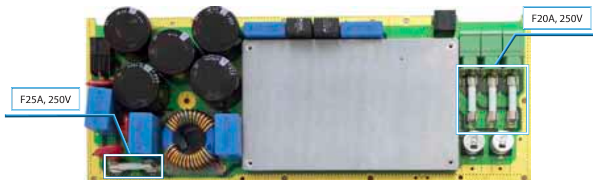
Figure A58 – Boxed Very High Power and pole-mount Remote Units: AC/DC Power Supply Module protection fuses position and electrical rating
