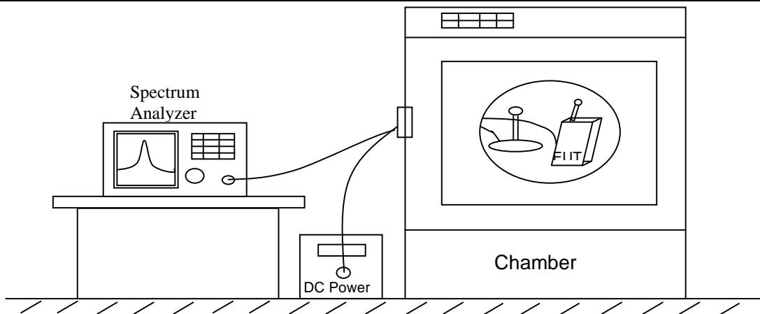
***Frequency stability measurement configuration***
