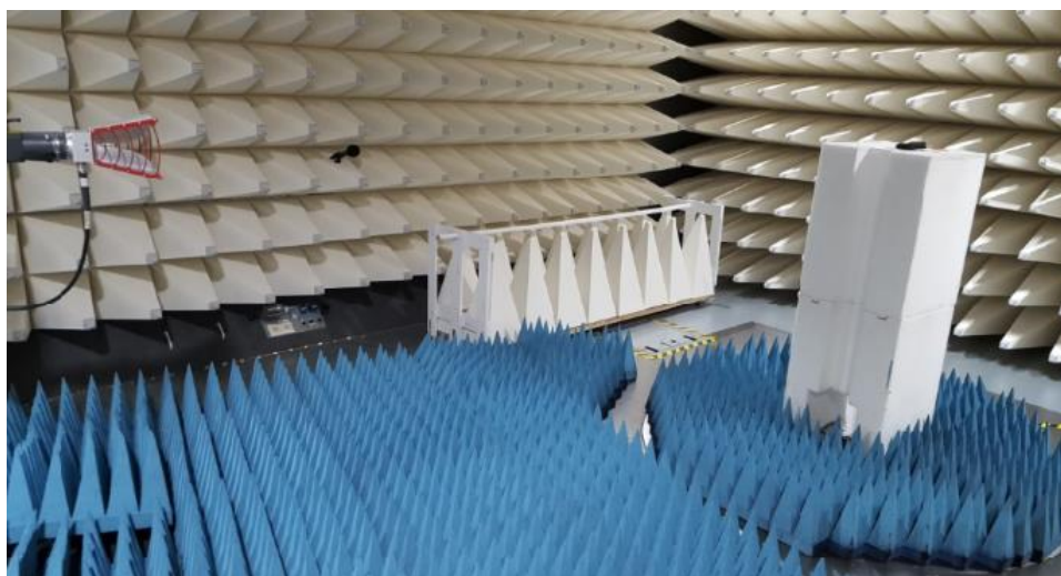
Figure B2. EIRP Radiated Test Setup
