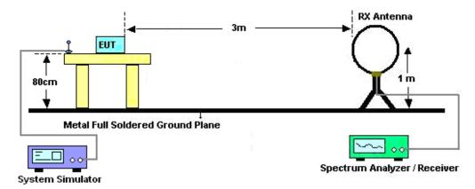
For radiated emissions from 30MHz to 1GHz
