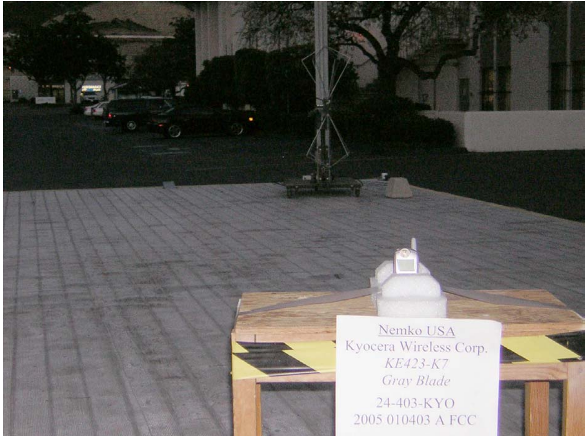
Photograph 2. FCC, Part 15 Radiated Emissions Test Configuration
