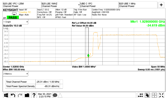
Figure 8.3-116: Conducted band edge emission at 1929 MHz, CDMA and LTE 20 MHz, antenna port B two-carrier operation (RBW = 1 MHz)
