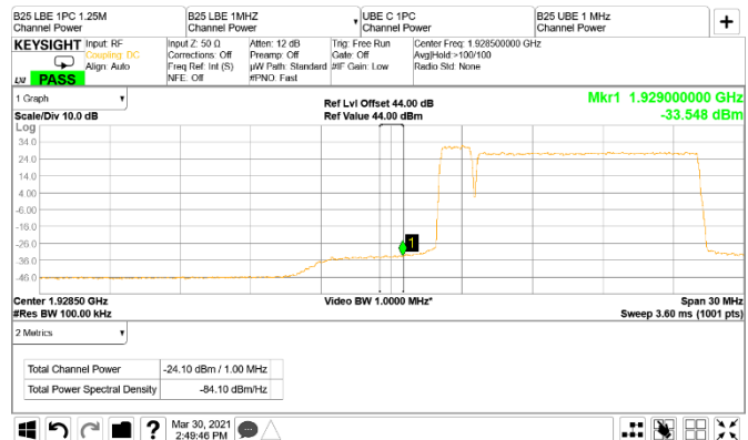
Figure 8.3-132: Conducted band edge emission at 1929 MHz, CDMA and NR 10 MHz, antenna port B two-carrier operation (RBW = 1 MHz)
