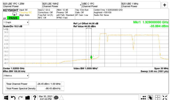
Figure 8.3-152: Conducted band edge emission at 1929 MHz, CDMA, LTE 5 MHz and NR 5 MHz, antenna port A three-carrier operation (RBW = 1 MHz)
