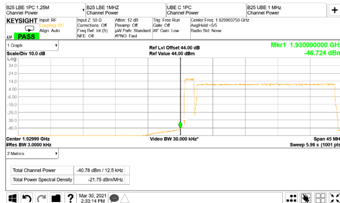
Figure 8.3-143: Conducted band edge emission at 1930 MHz, CDMA and NR 20 MHz, antenna port A two-carrier operation (RBW = 1% of EBW)
