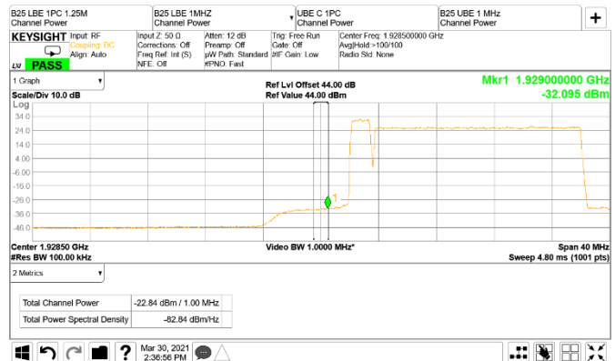
Figure 8.3-140: Conducted band edge emission at 1929 MHz, CDMA and NR 15 MHz, antenna port B two-carrier operation (RBW = 1 MHz)
