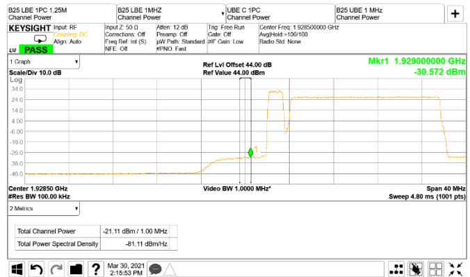
Figure 8.3-108: Conducted band edge emission at 1929 MHz, CDMA and LTE 15 MHz, antenna port B two-carrier operation (RBW = 1 MHz)
