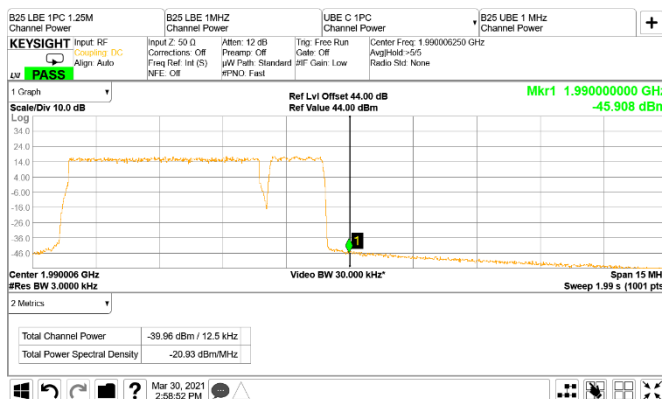
Figure 8.3-121: Conducted band edge emission at 1990 MHz, CDMA and NR 5 MHz, antenna port A two-carrier operation (RBW = 1% of EBW)
