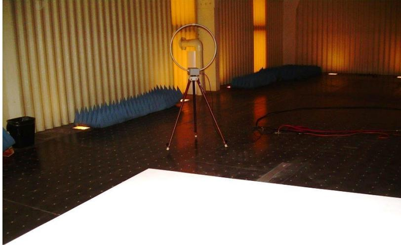
**Photograph 5: Loop Antenna Setup Used for Frequencies Below 30 MHz**
