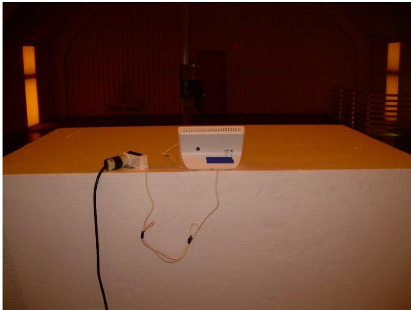
**Photograph 4: Back View Radiated Emissions Configuration – Below 1000 MHz**
