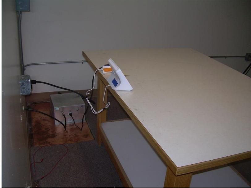
**Photograph 7 - Back View Conducted Emissions Worst Case Configuration**
