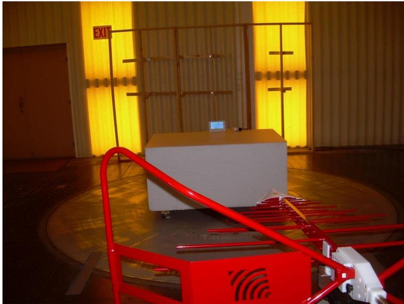
**Photograph 1: Front View Radiated Emissions Configuration – 30 – 1000 MHz**
