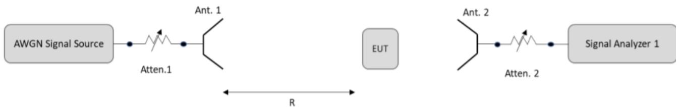
Figure 7-6. Contention-based protocol test setup, radiated method, detection threshold measurement
