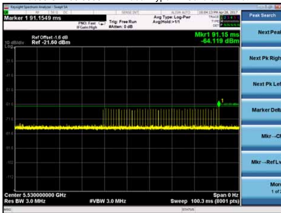
11ac80 CH106 5530MHz Radar Type 1B Calibration Plot
