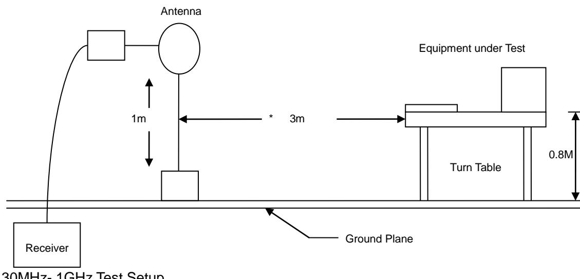
30MHz- 1GHz Test Setup
