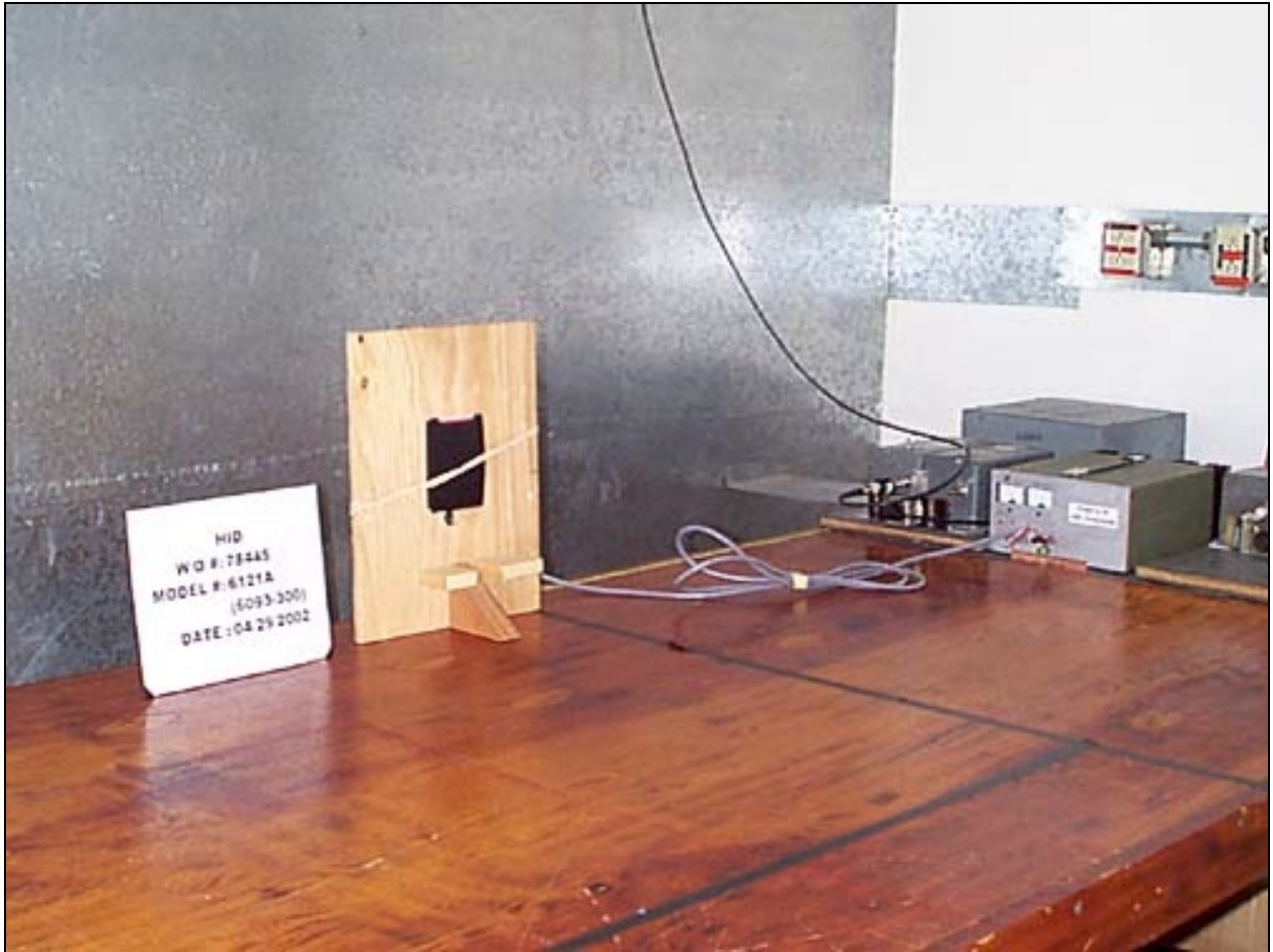
Mains Conducted Emissions - Front View - 6121A
