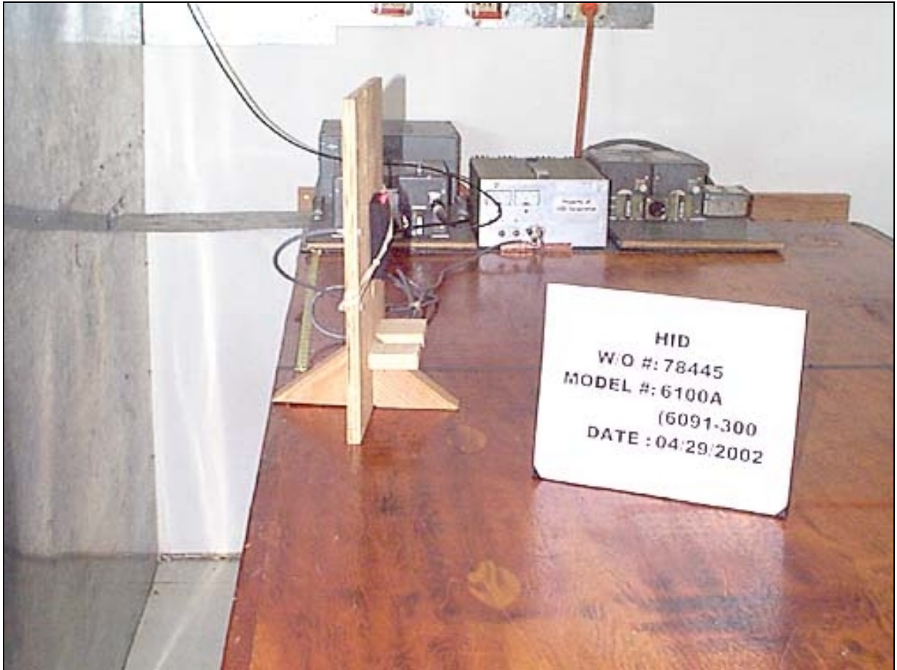
Mains Conducted Emissions - Side View - 6100A
