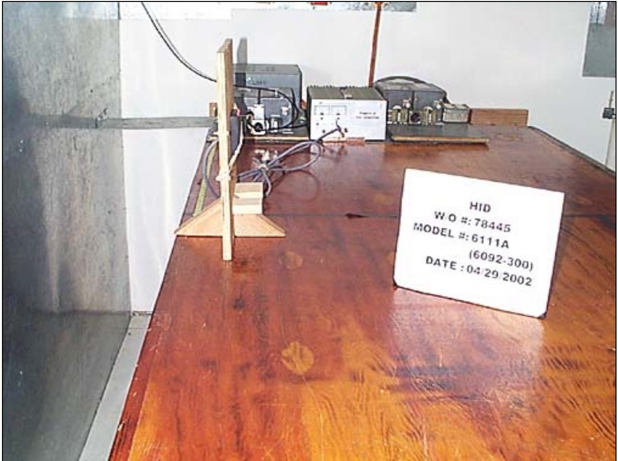
Mains Conducted Emissions - Side View - 6111A
