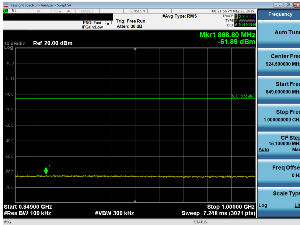
Plot 7-51. Conducted Spurious Plot (Band 5 - 3.0MHz QPSK - RB Size 1, RB Offset 0 - Low Channel)
