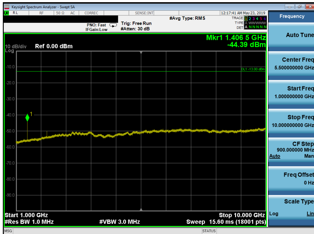
Plot 7-46. Conducted Spurious Plot (Band 12 - 10.0MHz QPSK - RB Size 1, RB Offset 0 - Mid Channel)
