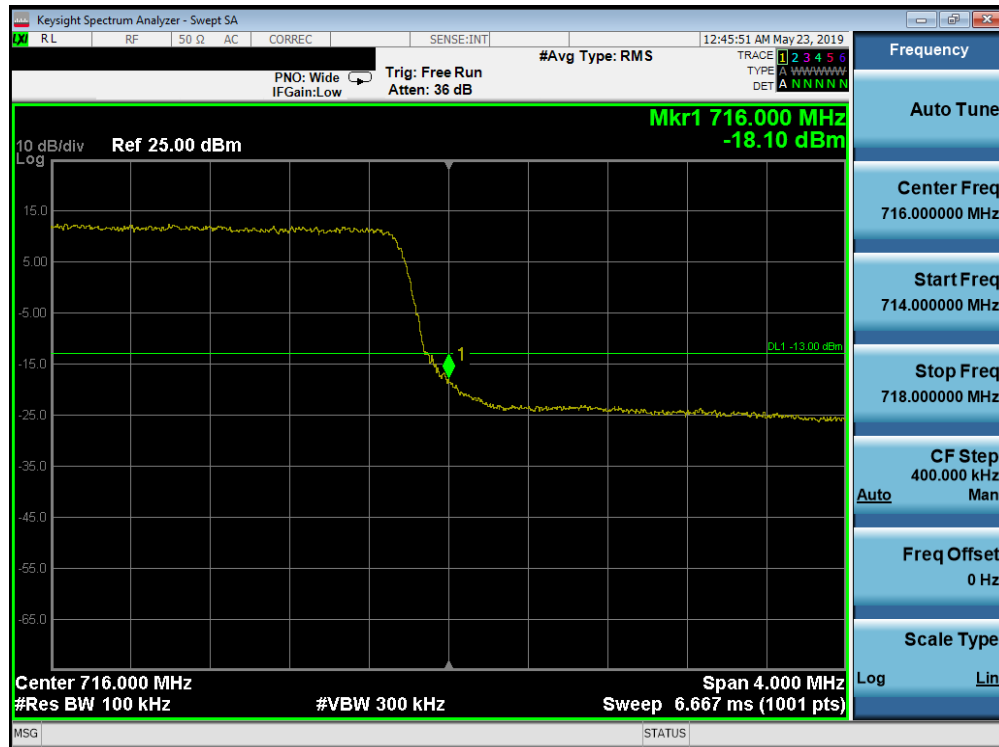
Plot 7-83. Upper Band Edge Plot (Band 12 - 5.0MHz QPSK - Full RB Configuration)
