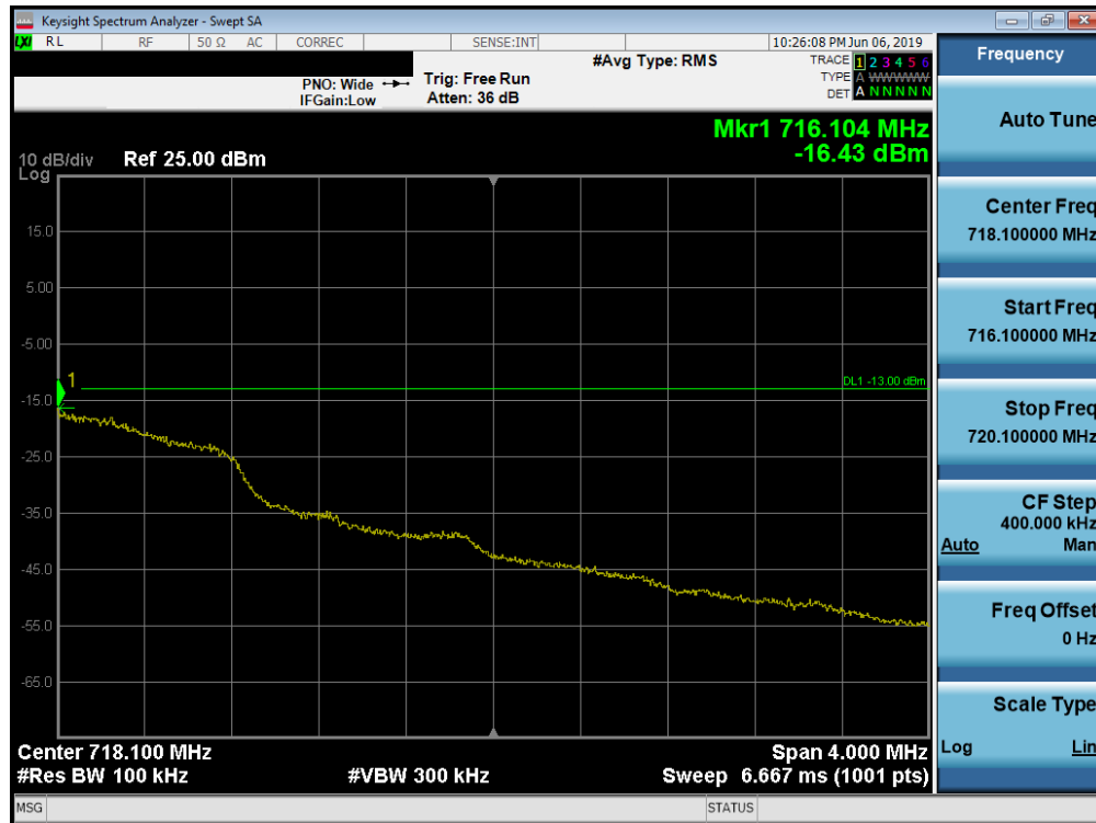
Plot 7-79. Upper Extended Band Edge Plot (Band 12 - 1.4MHz QPSK - Full RB Configuration)
