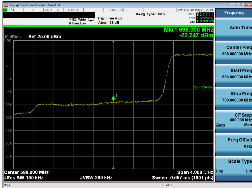
Plot 7-80. Lower Band Edge Plot (Band 12 - 3.0MHz QPSK - Full RB Configuration)
