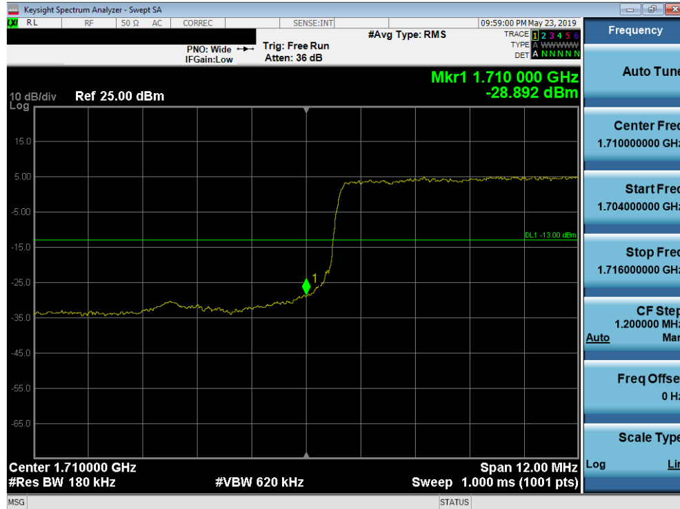
Plot 7-114. Lower Band Edge Plot (Band 4 - 20.0MHz QPSK - Full RB Configuration)
