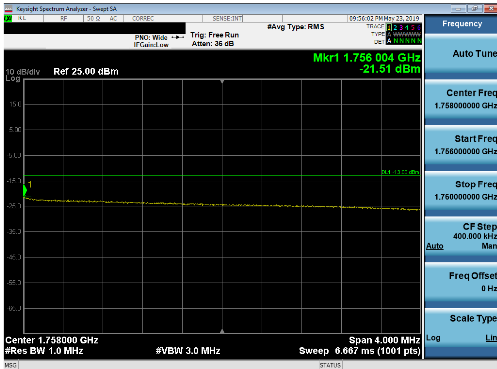
Plot 7-109. Upper Extended Band Edge Plot (Band 4 - 10.0MHz QPSK - Full RB Configuration)
