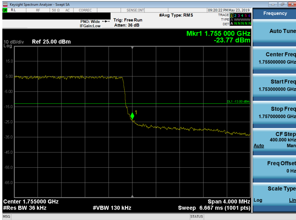
Plot 7-100. Upper Band Edge Plot (Band 4 - 3.0MHz QPSK - Full RB Configuration)
