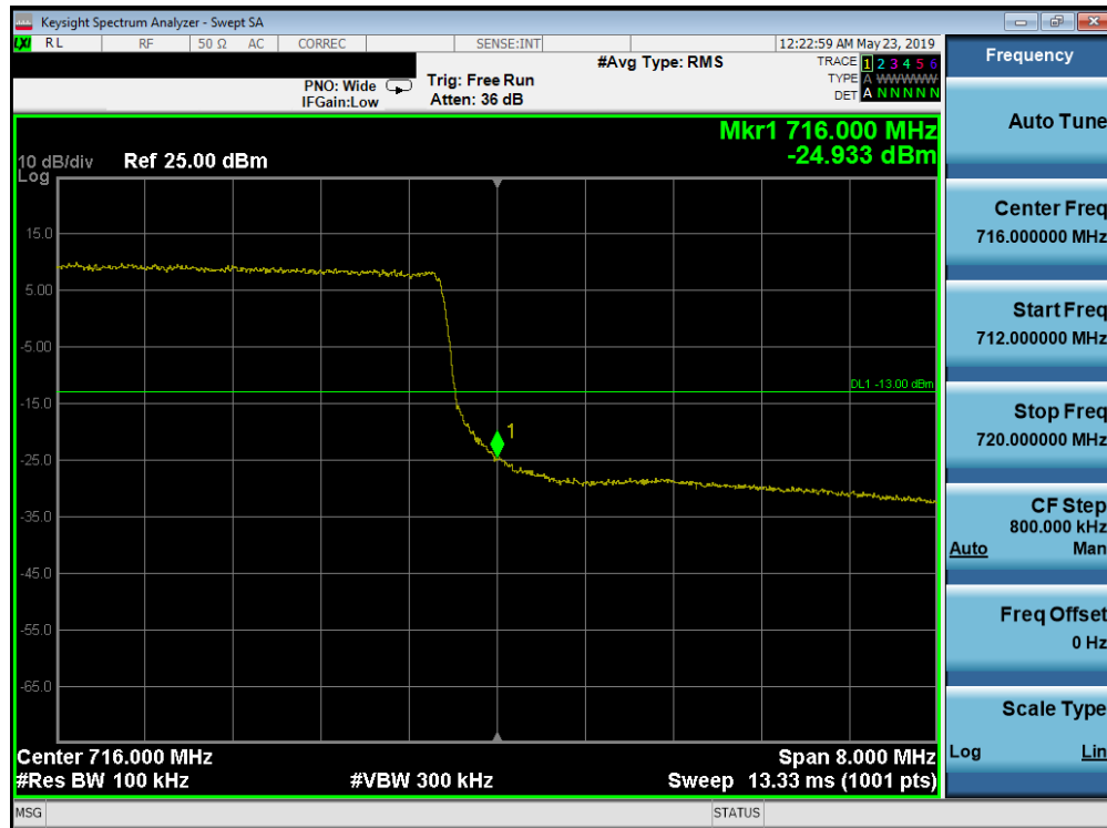
Plot 7-85. Upper Band Edge Plot (Band 12 - 10.0MHz QPSK - Full RB Configuration)
