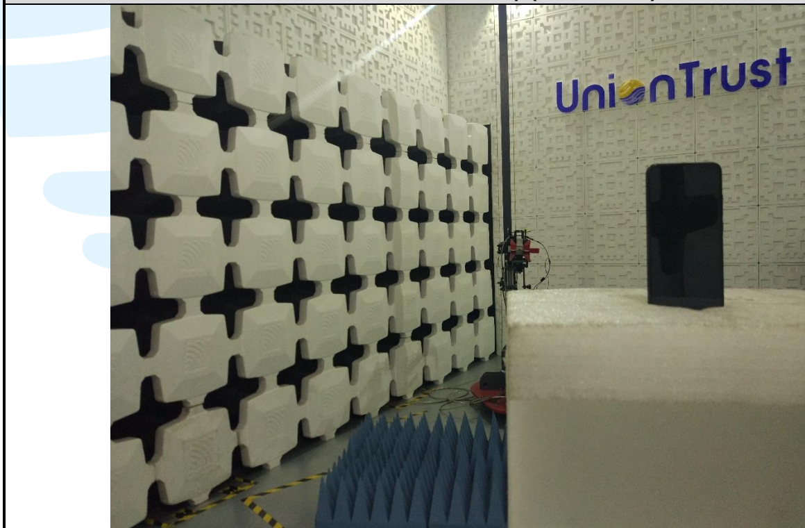
Radiated emission Test Setup (Above 1 GHz)
