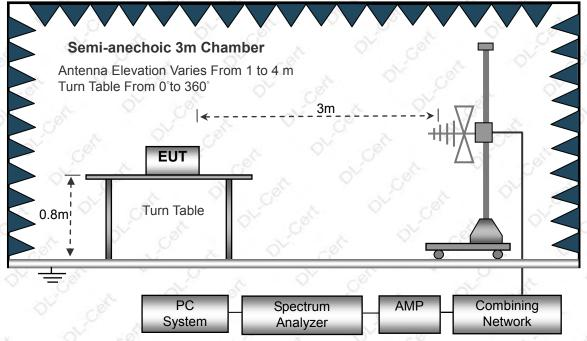
(C) Radiated Emission Test-Up Frequency Above 1GHz
