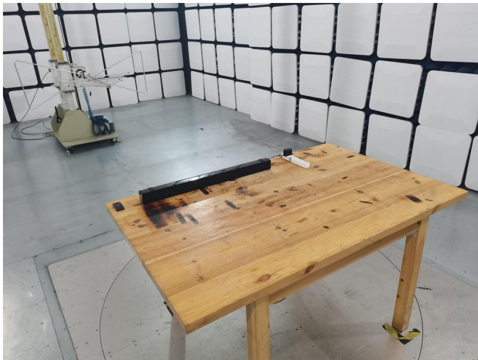
Photo of Radiation Emission Test
