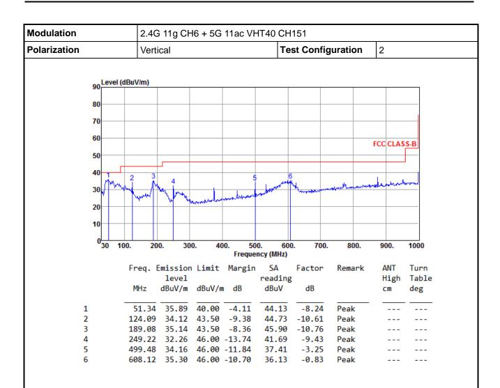
\*Factor includes antenna factor, cable loss and amplifier gain
