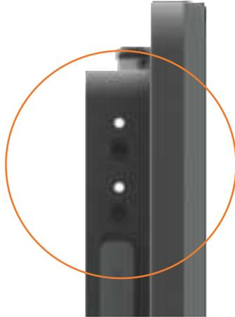
Switch ports S1 and S2 have an LED indicator above that illuminate when a switch is activated.
