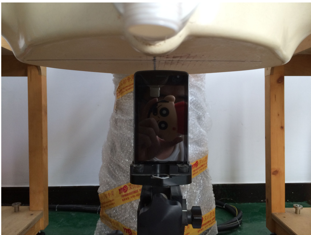
10mm Body-worn Top Side Setup Photo
