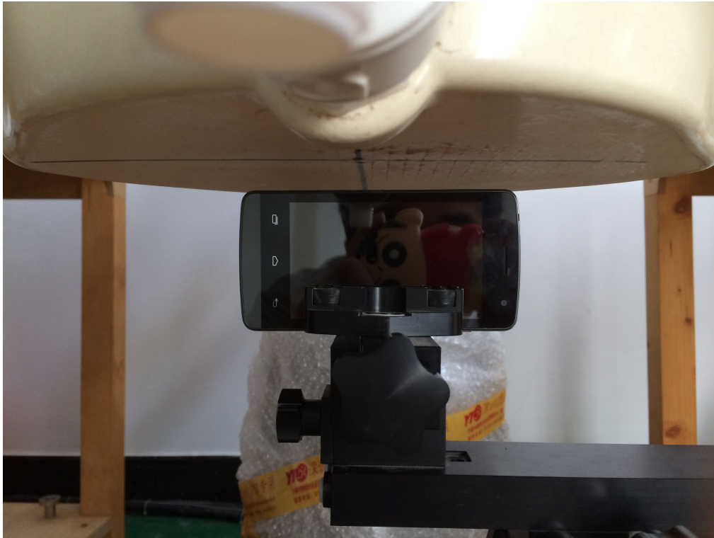
10mm Body-worn Right Side Setup Photo
