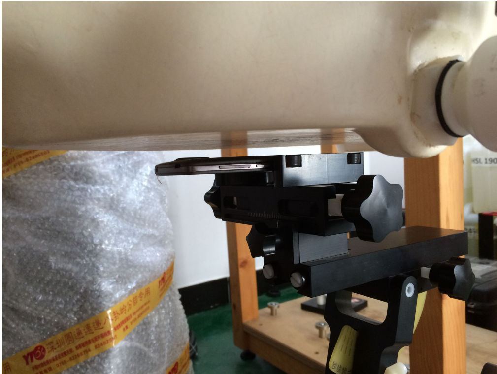
10mm Body-worn Rear Setup Photo
