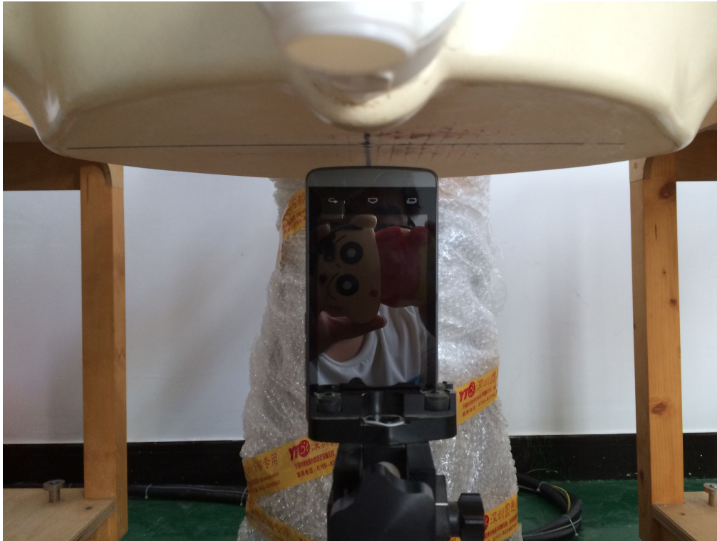
10mm Body-worn Bottom Side Setup Photo
