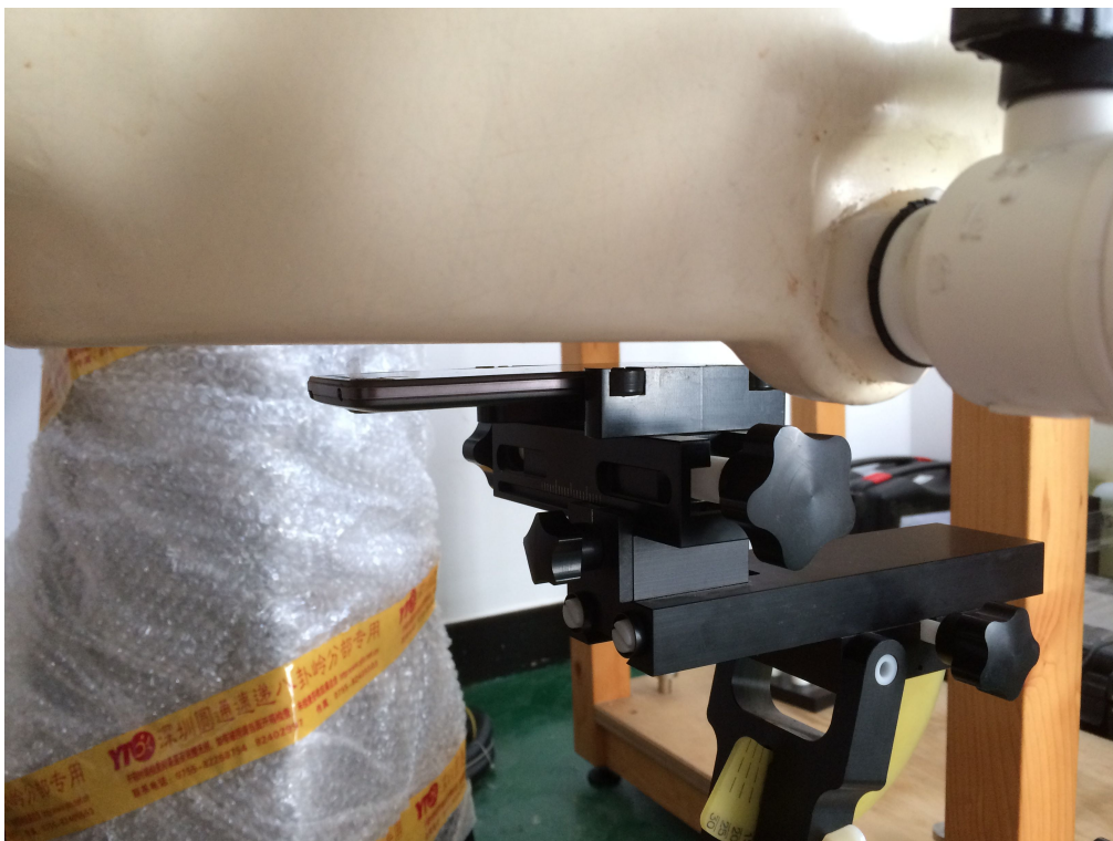
10mm Body-worn Front Side Setup Photo
