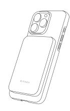
Note: Your phone will start charging automatically once attached to the power bank. Remove it to stop charging. No need to press any buttons.
