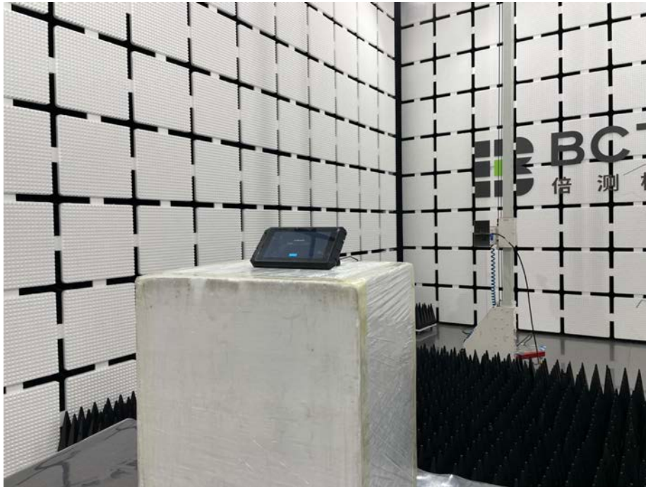
Spurious Emission Test Setup (above 1GHz)
