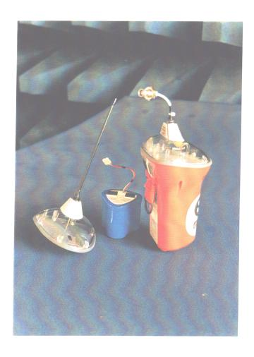
EPIRB (with test lead) alongside Antenna & Battery
