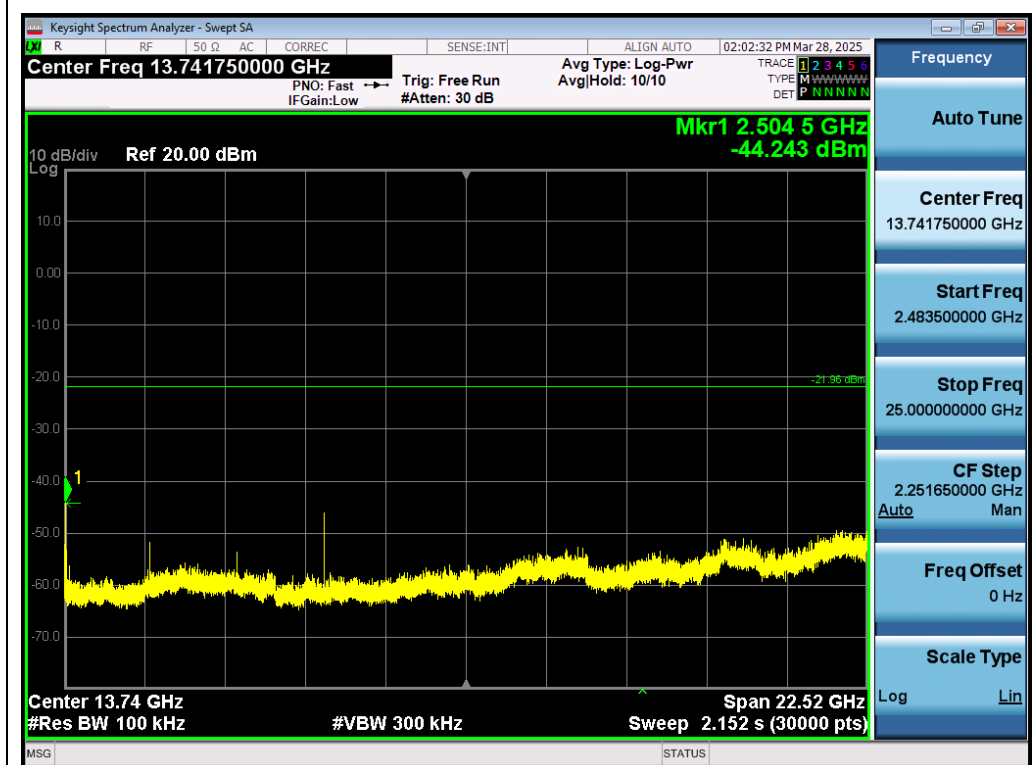
Test_Graph_LE1M_ANT1_2440_1Mbps_Higher Band Emissions
