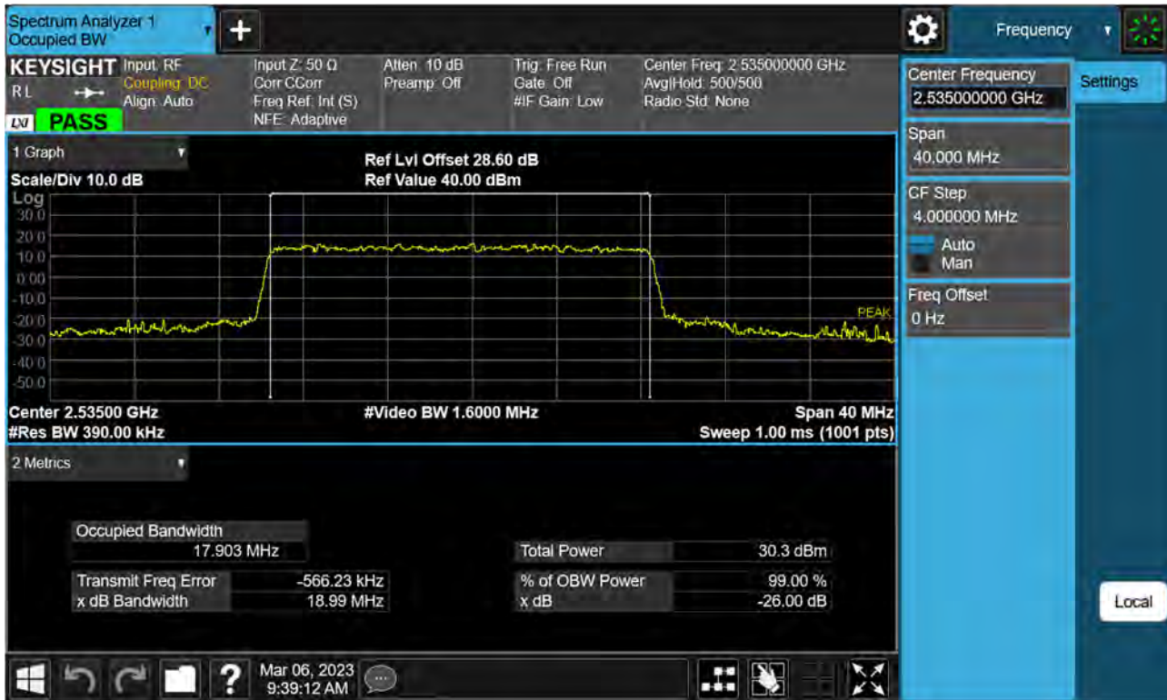
Sub6 n7. Occupied Bandwidth Plot (20 M BW Ch.507000 16QAM)
