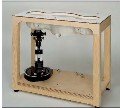
Picture C.10: SAM Twin Phantom
