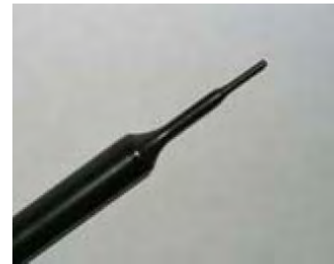
Picture C.2Near-field Probe
