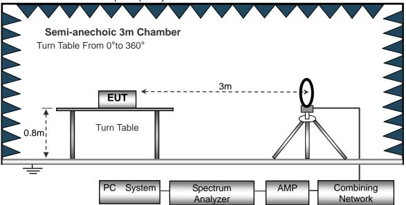
(B) Radiated Emission Test-Up Frequency 30MHz~1GHz
