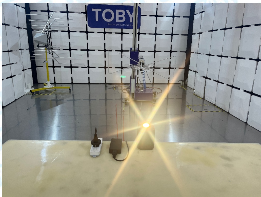
Photo of Setup for Radiated Emission (30MHz~1GHz)
