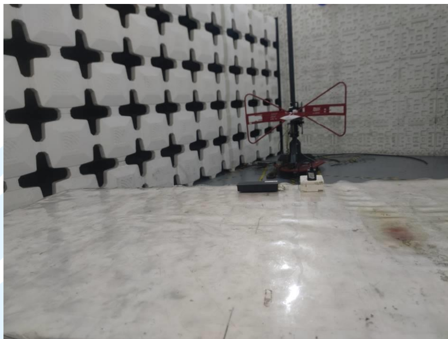
Radiated emission Test Setup-1 (30 MHz~1 GHz)
