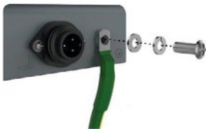
Connect Ground Cable at Rear Side
