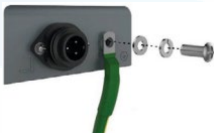
Connect Ground Cable at Rear Side
