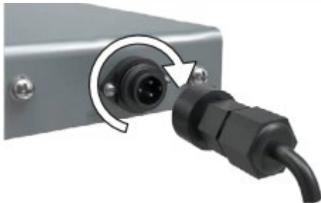
Connect Power Cable at Rear Side
