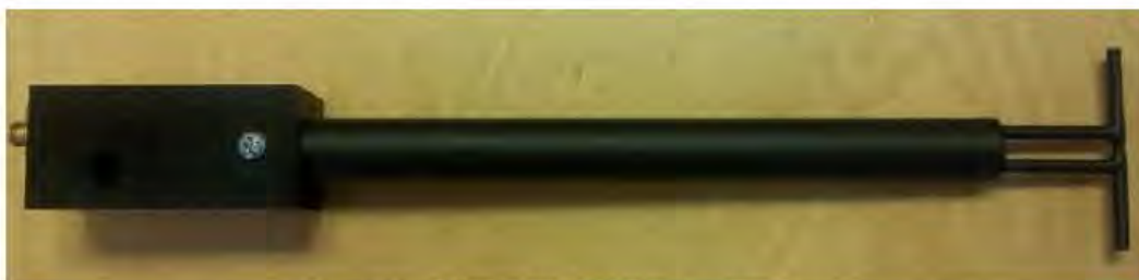
Figure 1 – MVG COMOSAR Validation Dipole
