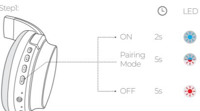
Press and hold it for 5s until the red and blue indicator lights flash alternately in power off mode. Turn on the Bluetooth of your device, and find "BLTD385" in the list to connect.
