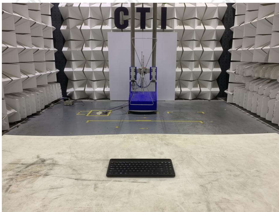
Radiated spurious emission Test Setup-1(Below 1GHz)
