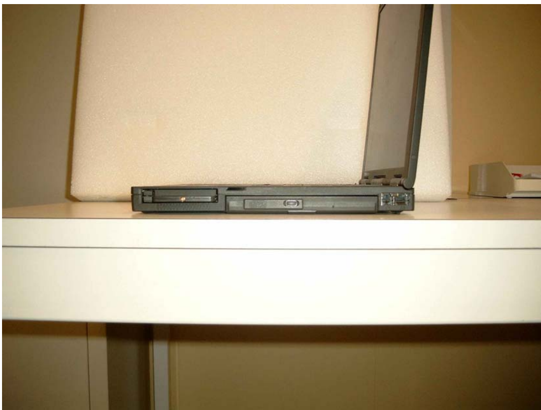
Figure 4 : Side view. Offset Card to base = 13 mm
