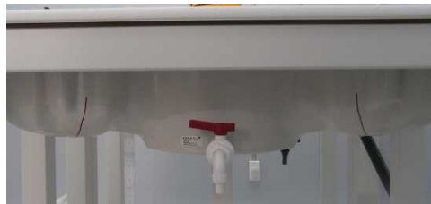
Figure 4.6 SAM Twin phantom
