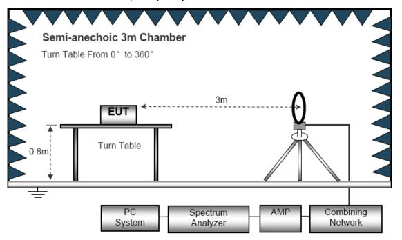
(B) Radiated Emission Test-Up Frequency 30MHz~1GHz
