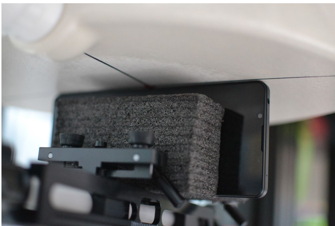
SAR Test Setup Photo 15 – Phablet, Left Edge at 0mm
