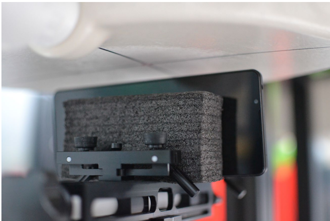
SAR Test Setup Photo 14 – Hotspot, Left Edge at 10mm
