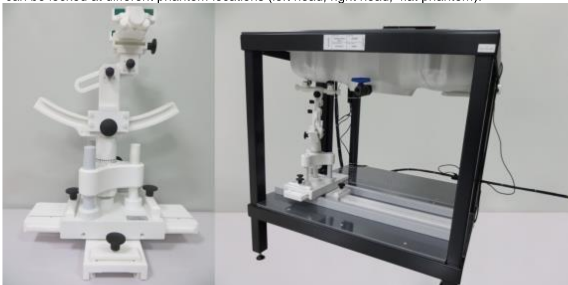
Device holder supplied by SATIMO
