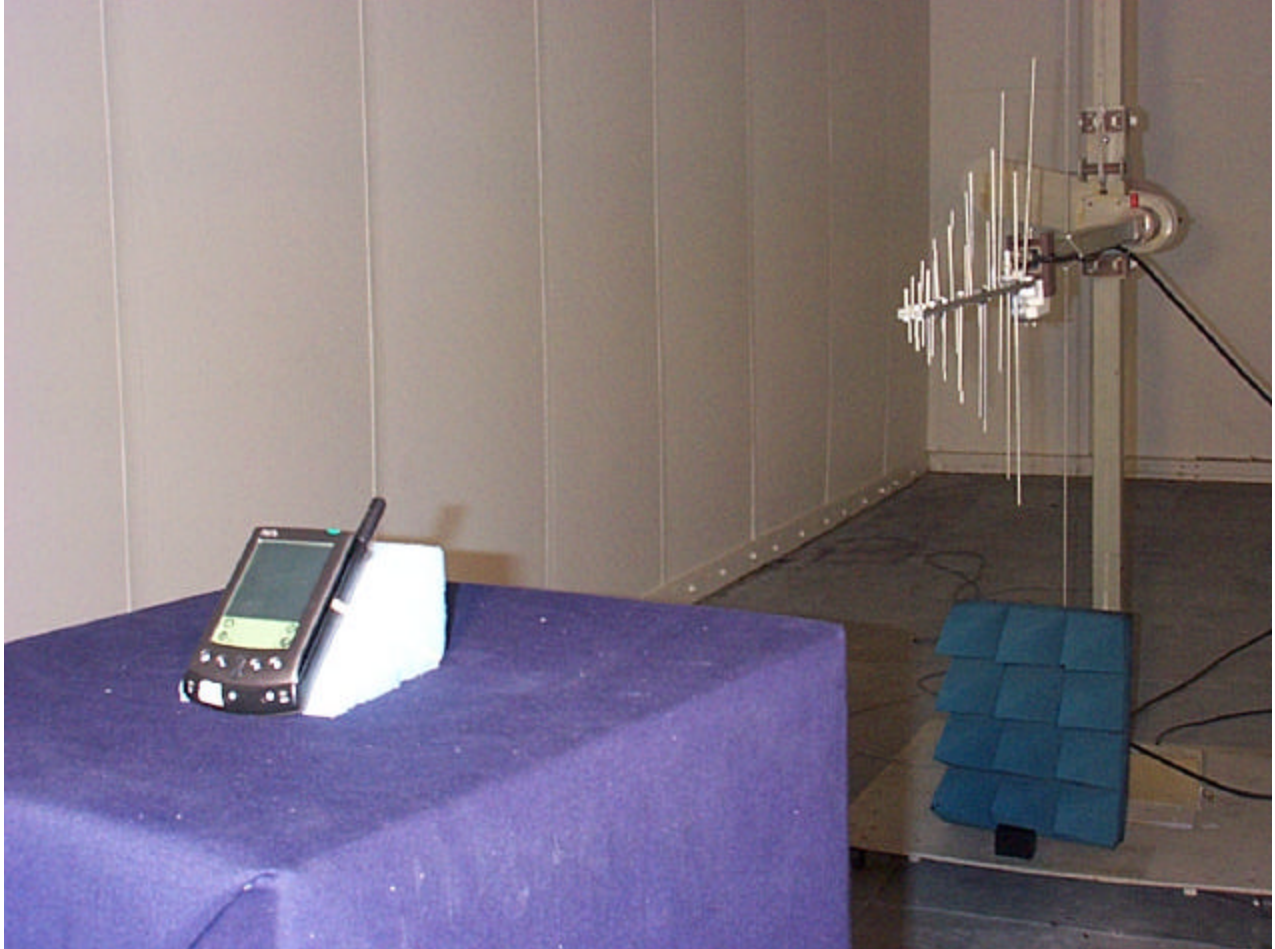
ERP Testing - 45° Tilt
